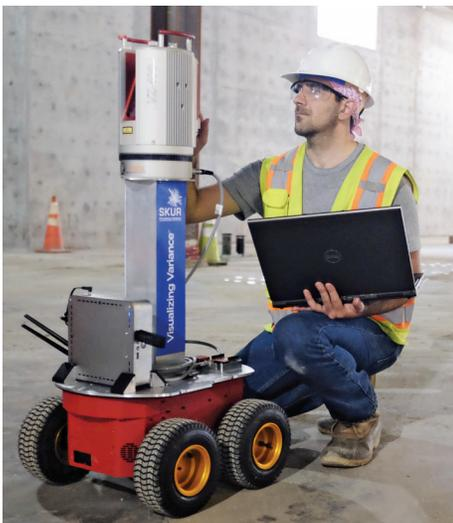
**SITE MAPPING** The SKURBOT sports a LiDAR unit to collect point-cloud data, but it is only a prototype.
